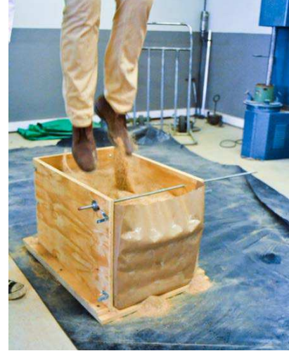
Applying a dynamic load during retaining wall test (competition by Geo Institute, ASCE)
